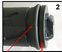
1 Typical tapered stub end with Bar Weight removed
