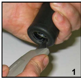
1 Cut 7/8" hole into ends of Stock Grips
